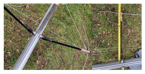
Measure spreader deflection by tensioning a string between the shrouds at the spreader and then measuring from the back of the mast track to the string.
