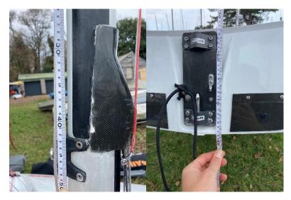
Hoist halyard and measure off at 6420mm at the top of the gooseneck. Then measure to lower edge of transom on the outside of the boat.
